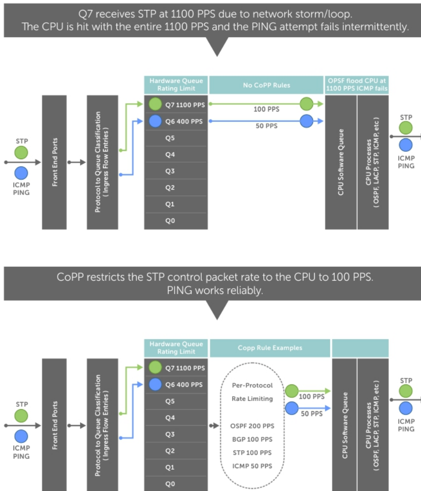
Figure 31. CoPP Implemented Versus CoPP Not Implemented
