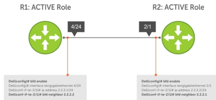
Figure 14. Establishing a BFD Session on Physical Ports
