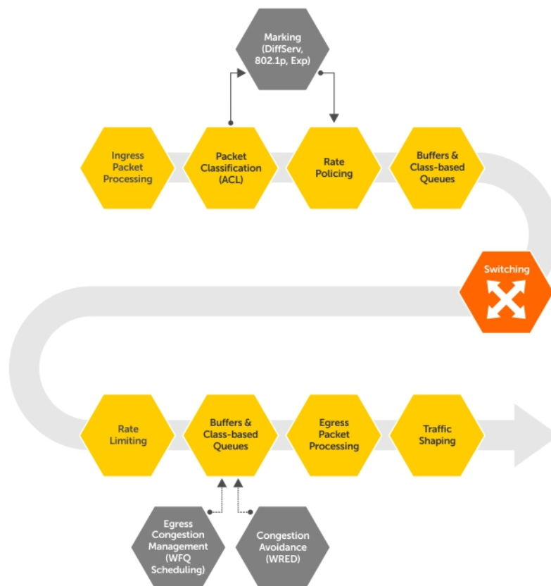
Figure 108. Dell EMC Networking QoS Architecture
