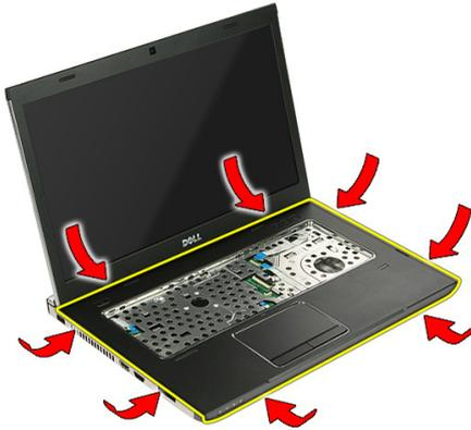
17. Lift up the palm rest from the computer and remove.
