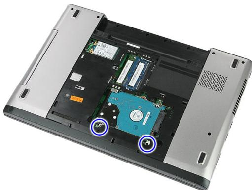
5. Lift up the hard drive at an angle from the system and remove.
