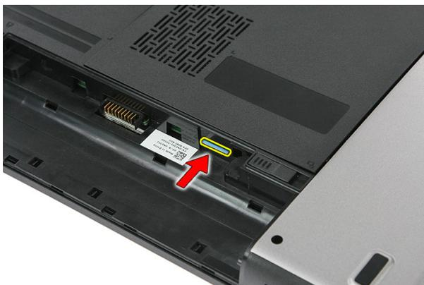
4. Grasp the SIM card and pull out to release it from the computer.
