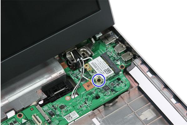
8. Remove the WLAN card from the computer.
