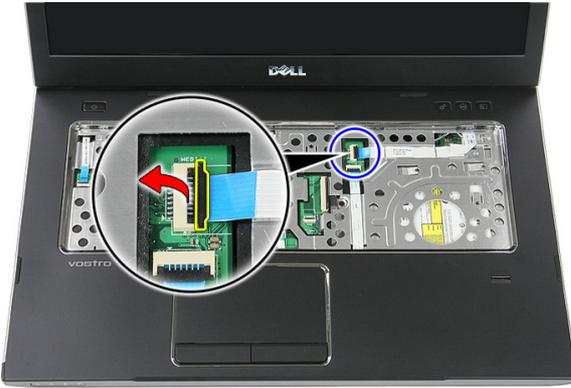
12. Disconnect the quick-launch button board cable.
