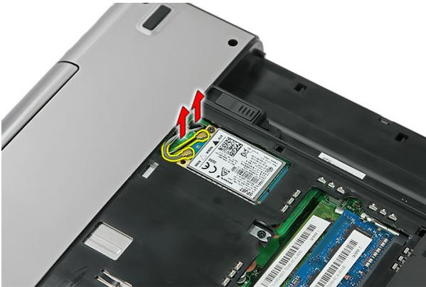
5. Remove the screw that secures the WWAN card.
