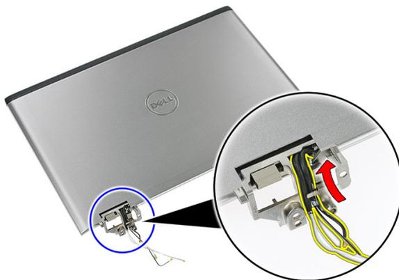
14. Remove the screws that secure the display brackets and hinges to the display assembly.
