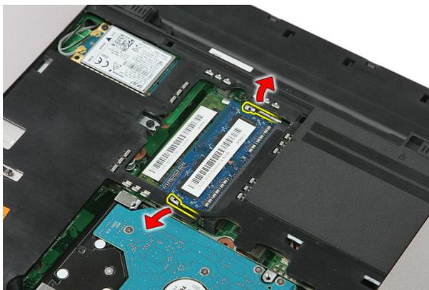
5. Remove the memory module from its connector on the system board.
