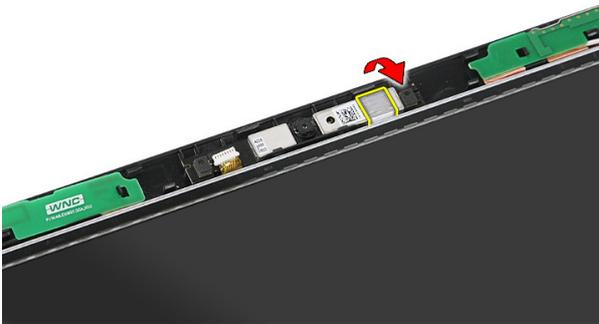
12. Pry the latch, then lift up the display and remove.
