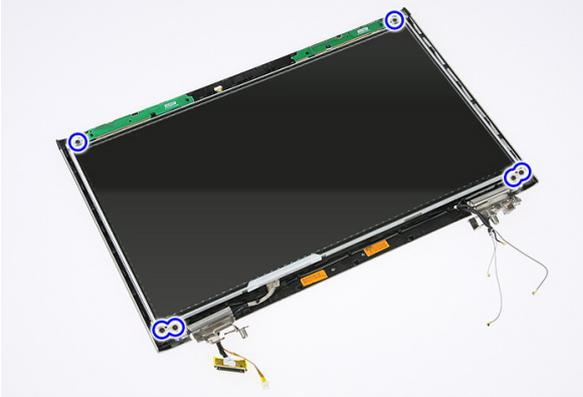
15. Lift up and remove the display panel with brackets and hinges.
