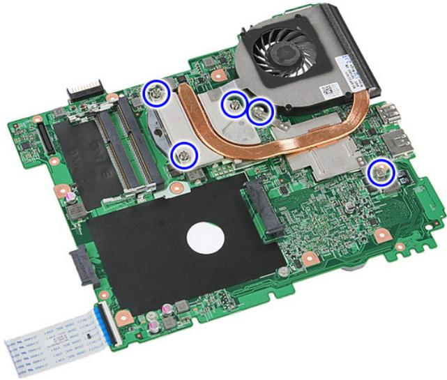
18. Lift up the heat sink and remove it from the system board.
