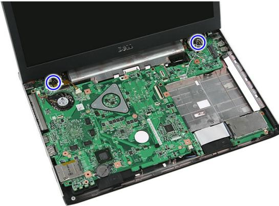
13. Lift the display assembly up from the system and remove.
