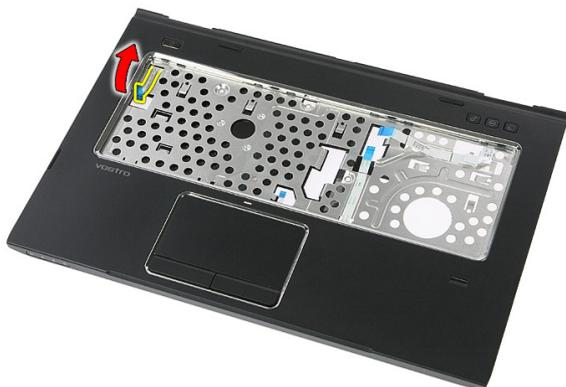
7. Remove the screw securing the power-button board.
