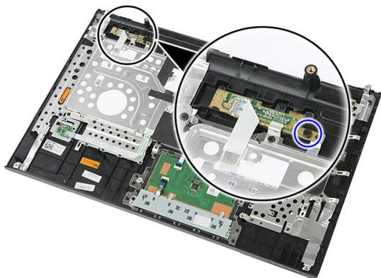
8. Lift up the quick-launch button board and remove.
