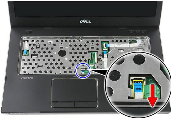
11. Release the quick-launch button board cable securing clip.
