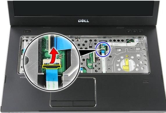
**14.** Disconnect the fingerprint-reader data cable.
