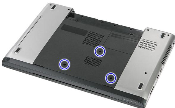
4. Lift the access panel up at an angle and remove it from the computer.
