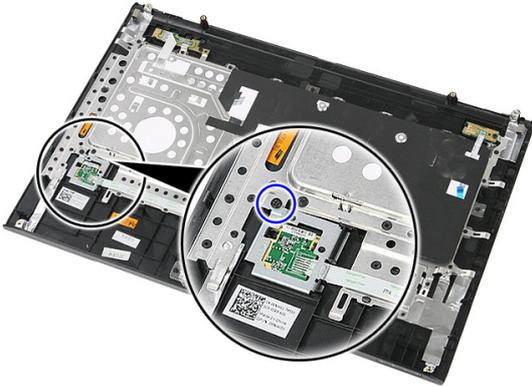
8. Lift up the fingerprint-reader bracket at an angle and remove.
