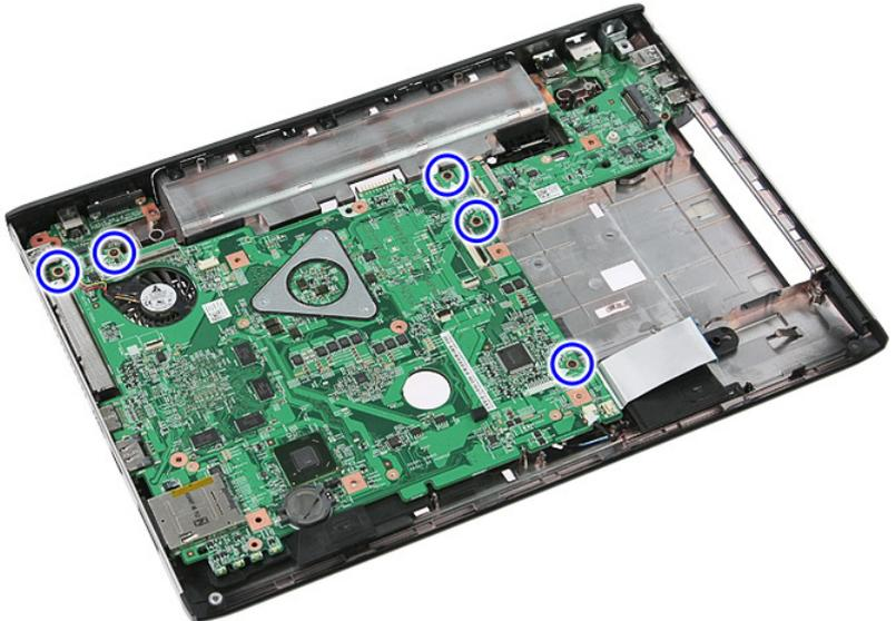
18. Lift up the system board at an angle and remove.
