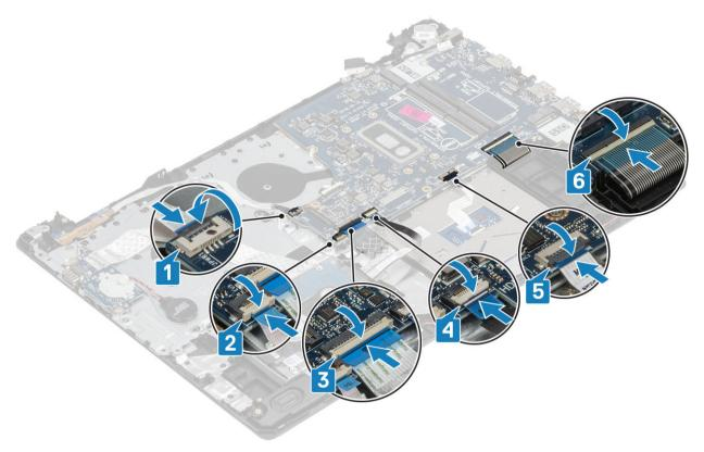
4 Connect the power adapter port cable and speaker cable to the system board [1, 2].
