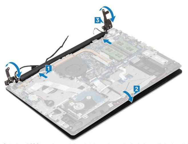
4 Replace the six (M2.5x5) screws that secure the left and right hinges to the system board, and palmrest and keyboard assembly [1].
