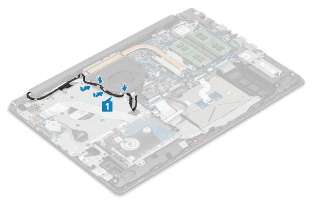
4 Connect the display cable and fan cable to the system board [1, 2].
