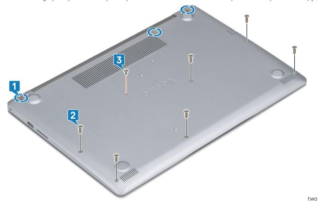
3 Pry the base cover from the top-left corner [1] and continue to pry open the sides of the base cover [2, 3, 4].
