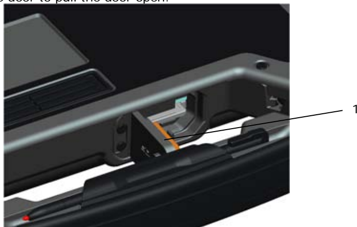
1 Secure digital door in its open position
