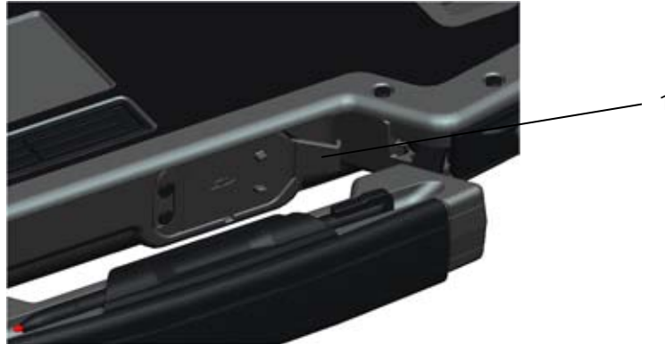
1 Secure digital door handle in extended position
