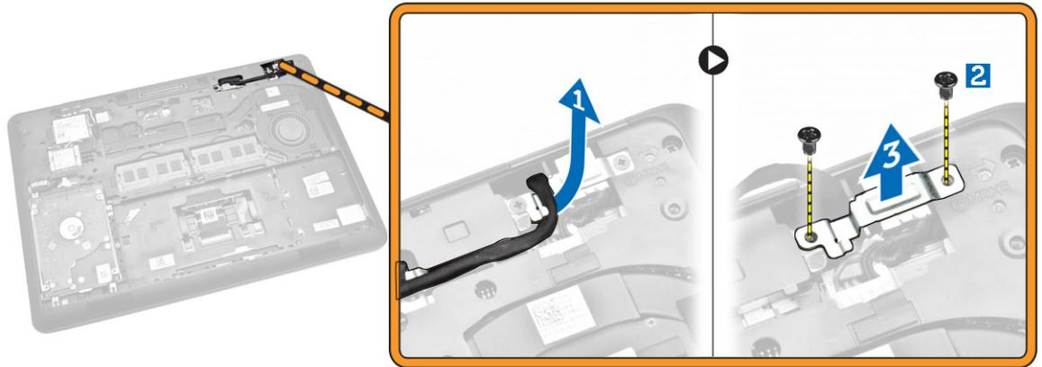
4. Disconnect the power-contractor port cable from its connector [1] and remove the power-contractor port from the computer [2].
