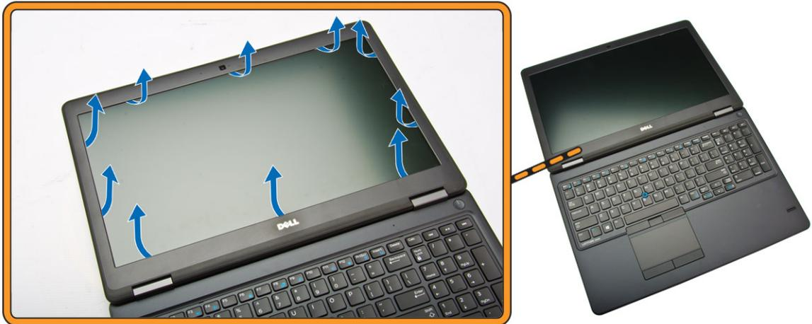
3. Remove the display bezel from the display assembly.
