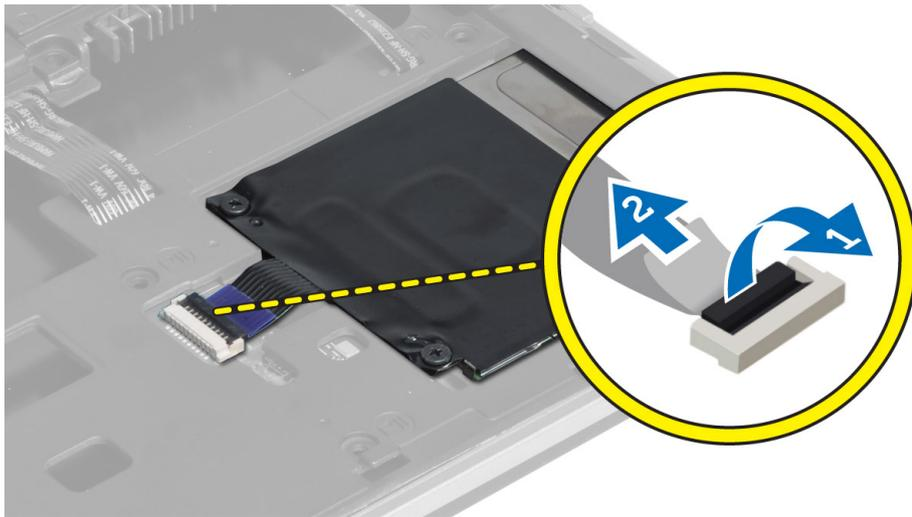
4. Remove the screws that secure the smart-card cage to the computer and remove it.
