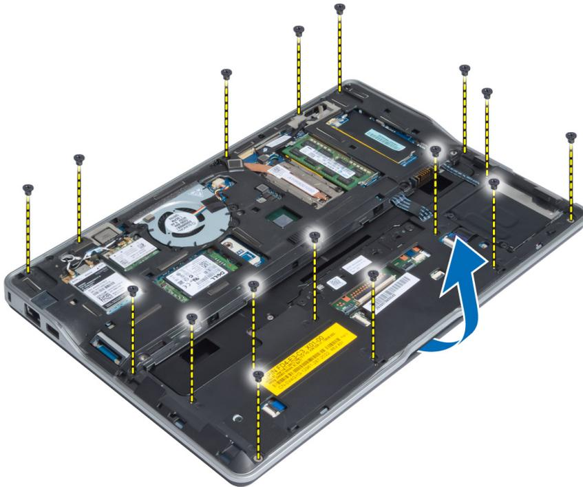
6. Press against the sections to release the palmrest assembly and remove it from the computer.
