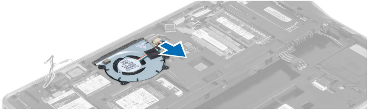
4. Disconnect the smart-card cable, hall-sensor cable and coin-cell battery cable.
