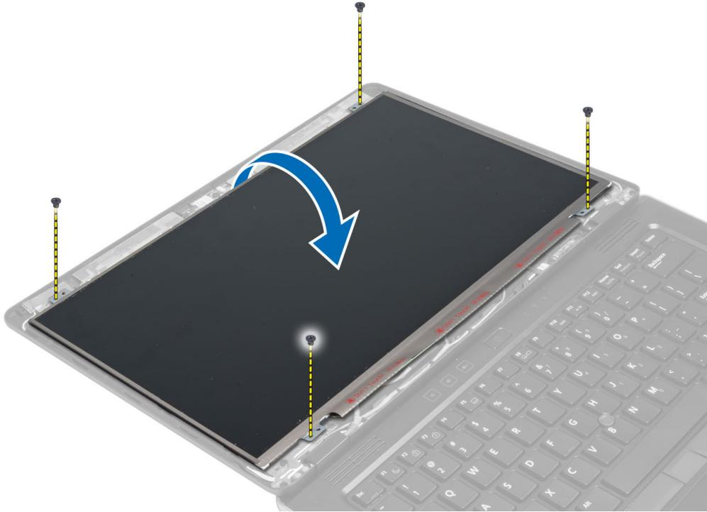
4. Peel off the LVDS cable connector tape and disconnect the LVDS cable from the display panel.
