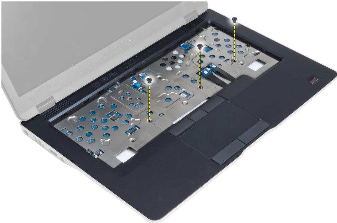
5. Flip the computer and remove the screws that secure the palmrest assembly to the base of the computer and flip open the lower assembly.
