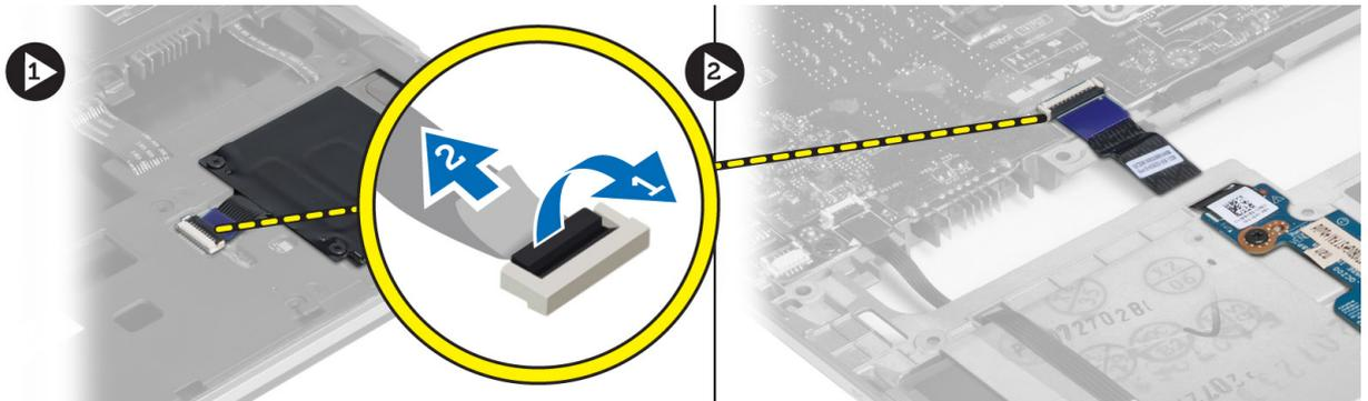
4. Remove the screws that secure the smart-card board in its place. Remove the smart-card cable from the routing channel and remove the smart-card from the computer.
