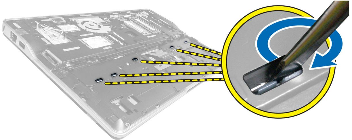
6. Flip the computer and remove the keyboard from the computer.
