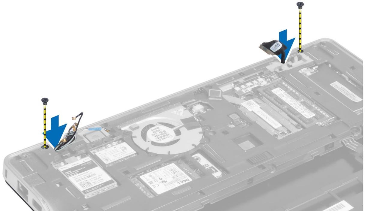
6. Remove the screws that secure the display assembly to the computer, and lift the display assembly from the computer.
