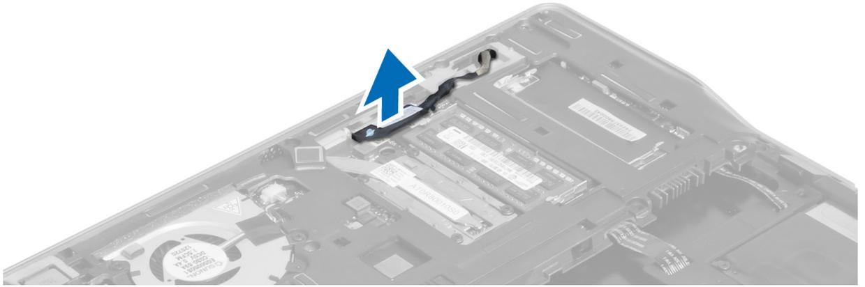
4. Disconnect the antenna cables from the wireless solution.
