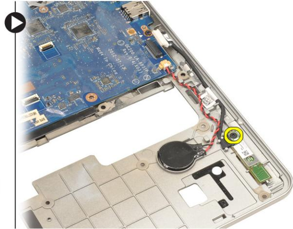
4. Remove the bluetooth card. Disconnect the cable from the card.
