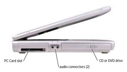
PC CARD SLOT — Supports one PC Card, such as a modem or network adapter. For more information, see "Using PC Cards" in the *Dell Latitude 100L Help* file. To access the help file, see page 16.
