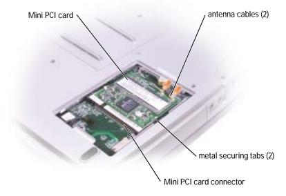
**NOTICE:** To avoid damaging the Mini PCI card, never place cables on top of or under the card.
