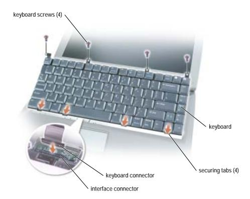
**9** Insert the four securing tabs on the keyboard into their respective slots in the palm rest, and lower the keyboard into the bottom case.
