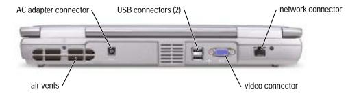
AIR VENTS — The computer uses an internal fan to create airflow through the vents, which prevents the computer from overheating.
