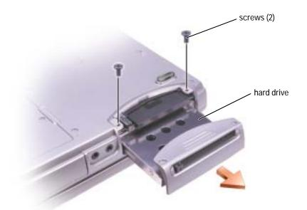
NOTICE: When the hard drive is not in the computer, store it in protective antistatic packaging. See
