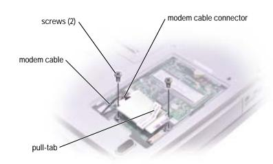
2 Connect the modem cable to the replacement modem.
