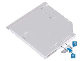
6 Pull the optical-drive bezel carefully to remove it from the optical drive.
