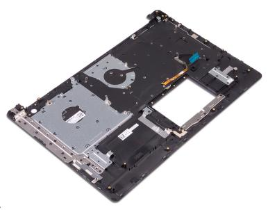
Place the palm rest and keyboard assembly on a flat surface.
