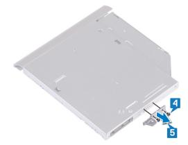
Pull the optical-drive bezel carefully to remove it from the optical drive.
