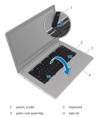
**3** Carefully turn the keyboard over and place it on the palm-rest assembly.
