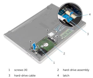
4 Disconnect the hard-drive interposer from the hard-drive assembly.
