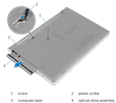
**3** Carefully pull the optical-drive bezel and remove it from the optical drive.
