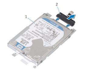
1 hard-drive assembly 2 hard-drive interposer
