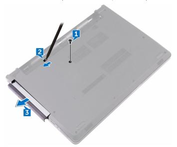
Remove the screw (M2x3) that secures the optical-drive bracket to the optical drive.
