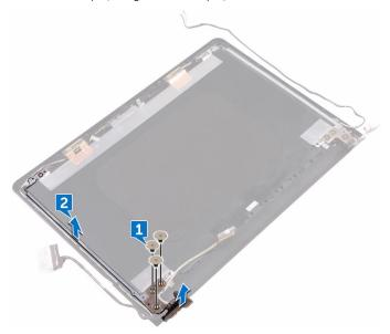
Note the display cable routing, and remove the display cable from the routing guides on the display back-cover and antenna assembly.
