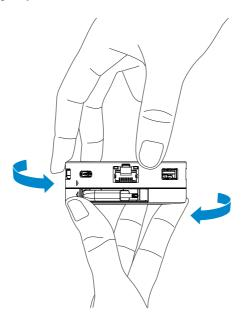
2. With the USB-C cable facing you, turn the top section to release the USB-C cable.
