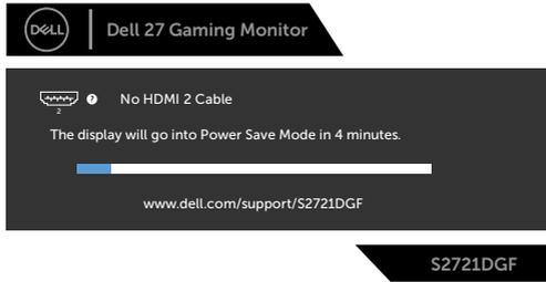
4. This box also appears during normal system operation if the video cable becomes disconnected or damaged.
