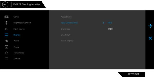
**Sharpness** Makes the image look sharper or softer. Move the joystick up and down to adjust the sharpness from '0' to '100'.
