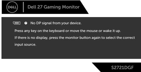
If either DP, HDMI 1 and HDMI 2 input is selected and the corresponding cable is not connected, a floating dialog box as shown below appears.
