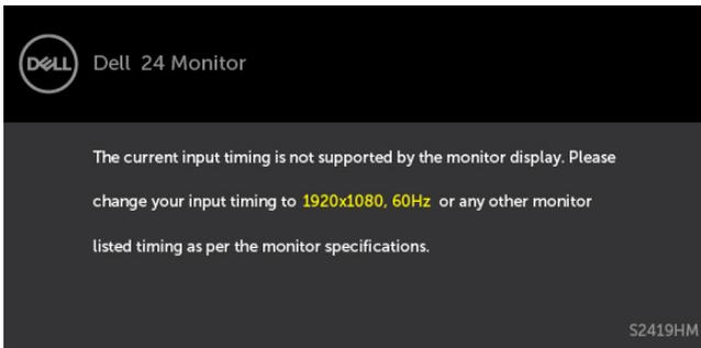
This means that the monitor cannot synchronize with the signal that it is receiving from the computer. See [Monitor Specifications](#) for the Horizontal and Vertical frequency ranges addressable by this monitor. Recommended mode is 1920 x 1080.
