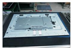
Put the rear cover with function key board into a Jip. Tear off the mylar tape on the function key board, then use a Philips-head screwdriver to tighten 3pcs screws for locking the function key board with the front bezel.
