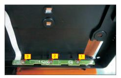
Tear off acetate tape, then disconnect the panel lamp cables from the connectors of the circuit board.
