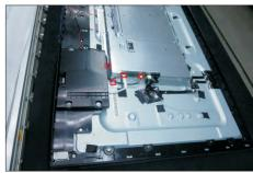
Use a Philips-head screwdriver to remove 2pcs screws for unlocking the heat-sink. Use a Philips-head screwdriver to remove 26pcs screws for unlocking the middle bezel, then remove the bezel.
