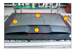
Lift the rear cover up carefully. Disconnect the USB LVDS cable and function key cable from the connectors of the interface board, and then remove the rear cover.
