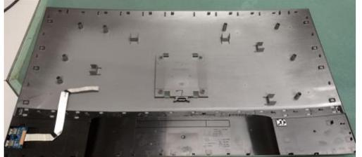
S5 Remove gasket from USB BD and unlock 1 screw to disassemble USB BD from RC
