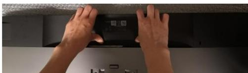
S4 Disassemble USB BD FFC cable from I/F BD first, then, take off RC from Middle frame
