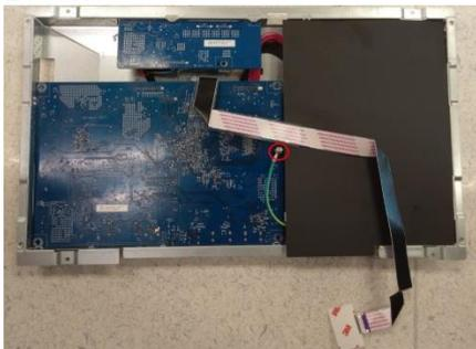
**S11** Unlock 6 screws and 1 earthing screw to disassemble PCBA from Bracket
