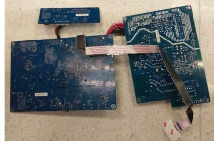
**S13** Unlock 3 screws to disassemble Control BD ASSY from Middle Frame
