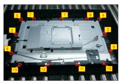
Disconnect the panel lamp from the connector of the panel, then release the panel lamp cable from the hooks of the middle bezel.
