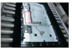
Use a Philips-head screwdriver to remove 13pcs screws for unlocking the middle bezel with the panel module.
