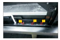
S15 Turn over the bracket chassis module. Remove the Mylar tape from the hooks of the bracket.
