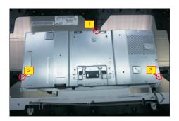
S11 Disconnect the panel power cable from the two connector of the panel module, then release the panel power cables from the hooks of the middle bezel.
