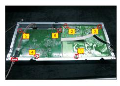
Remove the power board board and interface board from the bracket chassis module carefully, and then disconnect all of the cables.
