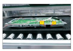
Remove the panel lamp cable from the hook of the bracket. Use a Philips-head screwdriver to remove 6pcs screws for interface board and power board. (No.1 screw size=M4x8, Torque=7±1kgfxcm; No.2~6 screw size=M3x7.5, Torque=7±1kgfxcm)
