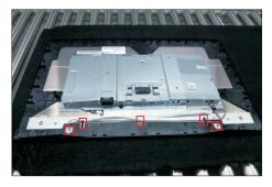
Move up the bracket, then push the earing-lock and disconnect the EDP cable away from the connector of the panel module.
