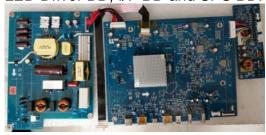
S25 Unlock 1 Grounding Screw and disassemble AC wire from Main SHD.
