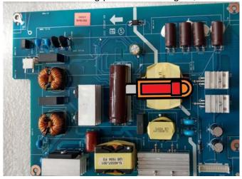
S26-3 Take out bulk cap. pin solder with soldering iron and absorber
