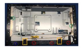
(TP-S Screw Torque: 6.5±0.5kgf) (FPH screw and base Screw Torque: 3.5~4.0kgf)
