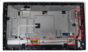
Remove long and short backlight wire from LED Driver BD.
