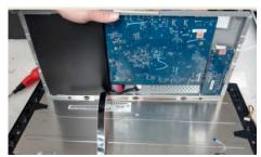
S17 Unlock 11 screws on Middle frame
