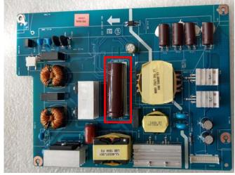
S26-1 Cut the glue between bulk cap. and PCB with a knife
