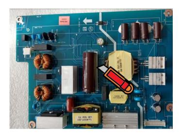
S26-2 Ensure cutting path within the glue, don't touch bulk cap. or PCB
