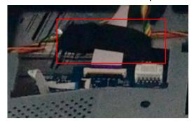
Remove USB FFC cable and USB wire from I/F BD.
