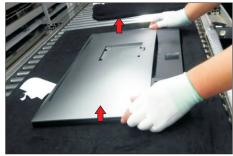
Remove the rear cover. Use a a Philips-head screwdriver to remove one screw for unlocking the USB unit, remove the USB unit from the hooks, and then disconnect the USB cable and function key cable away from the connectors of the circuit board. (No.1 screw size=M3x7.5, Torque=7~8kgfxcm)
