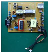
${\rm S1\,\, -1\,\, Cut}$  the glue between bulk cap. and PCB with a knife
