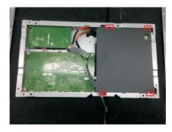
Use a Philips-head screwdriver to remove seven screws for interface board, LED driver board and S16 power board.
