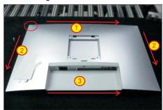
S7 Lift the rear cover up carefully. Disconnect the joystick key cable from the connector of the interface board, and then remove the rear cover and put it aside for later diasassembling.
