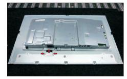
S17 Take away the bracket chassis module and then put the bracket chassis module on a protective cushion.
