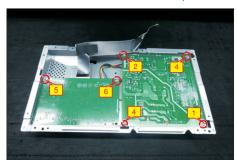
S17 Remove the circuit boards from the bracket chassis module carefully, and then disconnect all of the cables.
