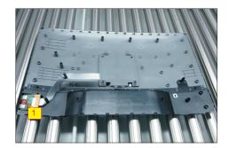
S8 Tear off 3pcs aluminium foils for unfixing the panel lamp cable.
