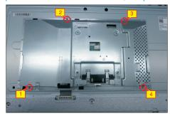
S14 Lift up the bracket chassis, and disconnect the LVDS cable from the connector of the panel module, then put the bracket chassis on a protective cushion.
