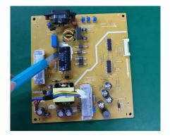
S1 -3 Cut into the bottom of bulk cap. and pull it up carefully
