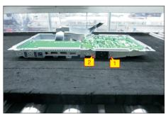
Use a Philips-head screwdriver to remove 6pcs screws for unlocking power board and interface board.
