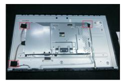
Use a proper tool to release the function key cable from the connector, then pull the function key cable high for releasing the function key cable as the picture below shown.
