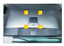
Wedge your fingers between the rear cover and the middle bezel on the corner of the top side of the monitor to release the rear cover, then use one hand to press the middle bezel, the other hand to pull up carefully the rear cover in order of arrow preference for unlocking mechanisms of rear cover.
