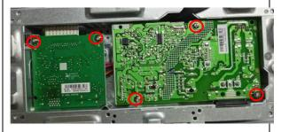
remove the screws on the board by the Philips-head. Torque=6±1kgf.c m
