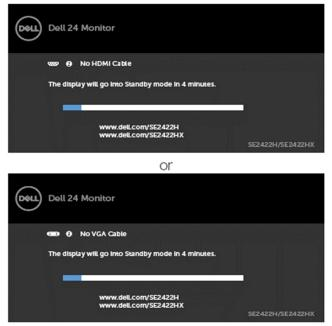
**NOTE:** This box also appears during normal system operation if the video cable is disconnected or damaged.
