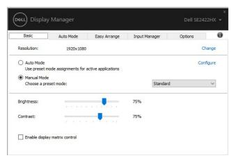
NOTE: When multiple Dell monitors are connected, select "Enable display matrix control" to apply brightness, contrast and color presets controls to all monitors.
