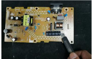
Lift the bulk cap. up and away from the PCB
