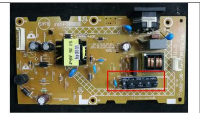
Remove electrolyte capacitors (red mark) from printed circuit boards
