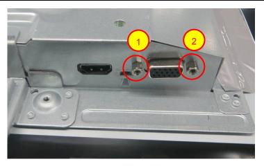
Use a hex screwdriver to remove 2 screws for unlocking mainboard.
