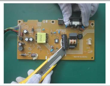
Lift the bulk cap. up and away from the PCB
