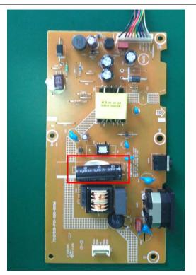
Remove electrolyte capacitors (red mark) from printed circuit boards
