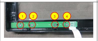
Use a Philips-head screwdriver to remove 4 screws for unlocking Key board.
