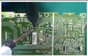
Take out bulk cap. pin solder with soldering iron and absorber
