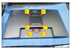
Turn over the LCD monitor to let the screen faced up, place a cloth on the panel where you are working on to protect the panel. Continually, wedge your fingers between the front bezel and the panel in order of arrow preference for unlocking mechanisms. Turn over the LCD monitor to let the screen faced down and then remove the rear cover.
