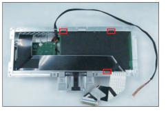
Use a Philips-head screwdriver to remove 4pcs
