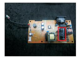
S16-1 Cut the glue between bulk cap. and PCB with a knife.
