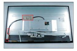
Use a Philips-head screwdriver to remove 2pcs screws for unlocking the bracket with panel module. Use a Hex-head screwdriver to remove 2pcs screws for unlocking the VGA connector.
