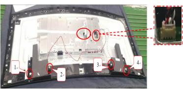
Use a Philips-head screwdriver to remove 4 screws for unlocking the speakers.
