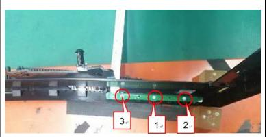
Use a Philips-head screwdriver to remove 3 screws for unlocking the key board
