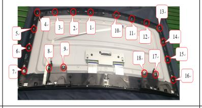
Use a Philips-head screwdriver to remove 18 screws for unlocking the middle frame (No.1~18 screw size=M3x4, Torque=3±0.5kgfxcm)
