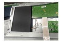
S6. Remove the main board and power board
