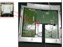
Use a Philips-head screwdriver to remove 4 screws for unlocking the main frame
