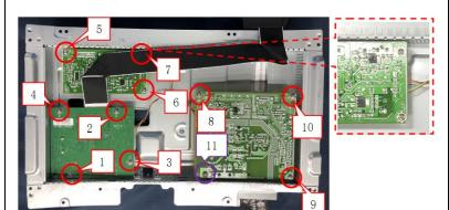
Use a Philips-head screwdriver to remove 11 screws for unlocking the main board and power board.
