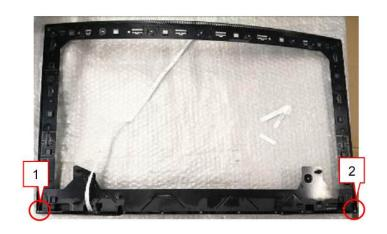
Use a Philips-head screwdriver to remove 2 screws for disassembling the deco bezel.
