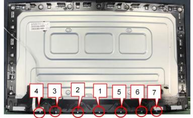
Use a Philips-head screwdriver to remove 7 screws to remove the DECO BEZEL.
