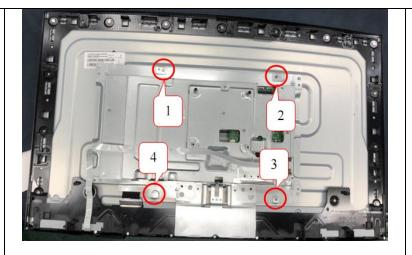
Use a Philips-head screwdriver to remove 4 screws for unlocking the main frame.
