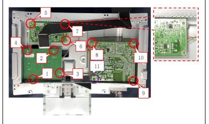
Use a Philips-head screwdriver to remove 11 screws for unlocking the main board and power board
