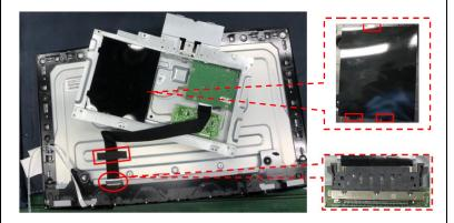
Turn over the mainframe, tear off tape and disconnect the FFC cable. Remove the mylar.
