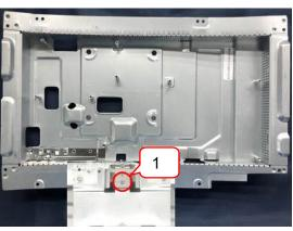
Use a Philips-head screwdriver to remove 1 screw for removing the stand\_button from main frame.
