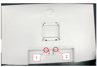
Use a Philips-head screwdriver to remove 2 screws for unlocking mechanisms.
