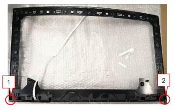
Use a Philips-head screwdriver to remove 2 screws for disassembling the deco bezel.
