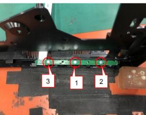
Use a Philips-head screwdriver to remove 3 screws for unlocking the key board.
