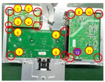
Use a Philips-head screwdriver to remove 12 screws for unlocking main board, power board, connect board (No.1~11 screw size=D3x6;
