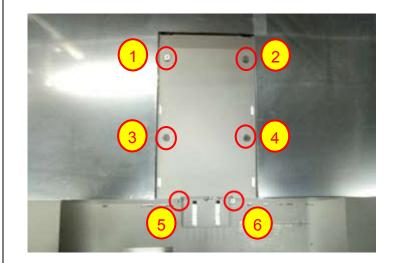
Use a Philips-head screwdriver to remove 6 screws for unlocking mechanisms.
