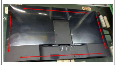
Use Penknife to separate the bezel and rear cove follow the arrows in sequence, then you can take out rear cover.
