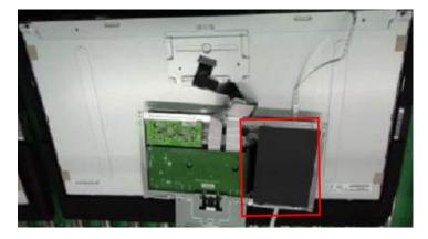
Remove the screws and the mylar.
