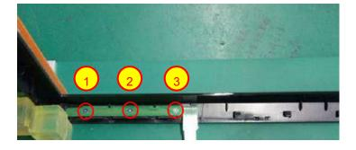
Use a Philips-head screwdriver to remove 3 screws for remove key board (No.1~3 screw size=M2x2.5; Torque=0.9±0.4kgf.cm)
