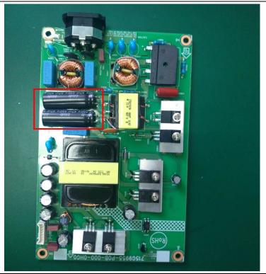
Remove electrolyte capacitors (red mark) from printed circuit boards
