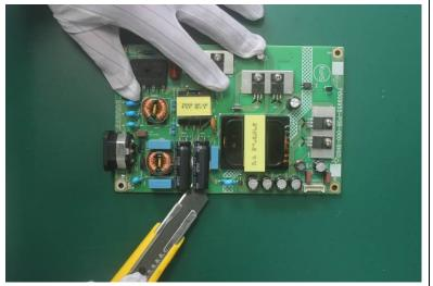
Lift the bulk cap. up and away from the PCB
