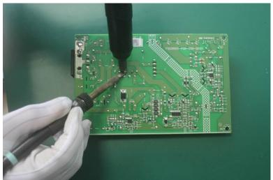
Take out bulk cap. pin solder with soldering iron and absorber
