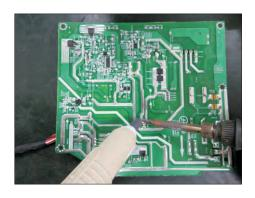
S22-5 Lift the bulk cap. up and away from the PCB.
