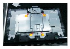
S10 Disconnect two LVDS cables and 1pcs panel lamp cable away from the connectors of the panel module, then take away the bracket chassis module and then put the bracket chassis module on a protective cushion.
