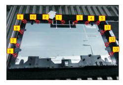
Tear off the Mic cable away from the panel, and then S15 lift up the middle bezel, then put it on a cushion foam for later disassembling.
