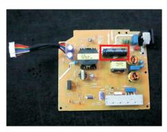
S22-1 Cut the glue between bulk cap. and PCB with a knife.
