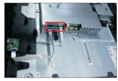
Disconnect the connective cable from the connector of the connect board, then use a Philips-head screwdriver to remove one screw for unlocking the connect board, then release the connect board from the hooks of the camera unit. Use a Philips-head screwdriver to remove 4pcs screws for unlocking the bracket chassis module with the panel module.
