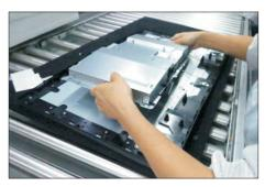
Use a Philips-head screwdriver to remove 1pcs screw for unlocking the USB board with middle bezel, then release the Usb board from the hooks of the middle bezel. Use a Philips-head screwdriver to remove 2pcs screws for unlocking the middle bezel with front bezel. Tear off the tape to release the camera connective cable from the panel.
