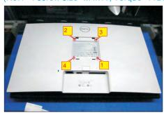
Wedge your fingers between rear cover and the middle bezel on the corners of the top side of the monitor to release the rear cover, then use one hand to press the middle bezel, the other hand to pull up carefully the rear cover in order of arrow preference for unlocking mechanisms of rear cover. Remove the rear cover and put it aside.
