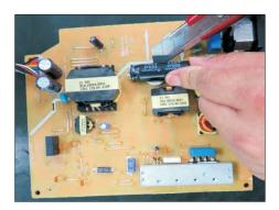
S22-3 Cut into the bottom of bulk cap. and pullit up carefully.
