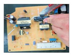
S22-4 Take out bulk cap. pin solder with soldering iron and absorber.
