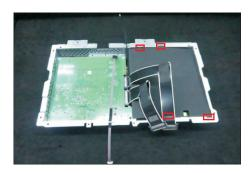
Use a Philips-head screwdriver to remove 7pcs screws for interface board and power board. Release the connective cable and panel lamp cable from the hooks of the bracket
