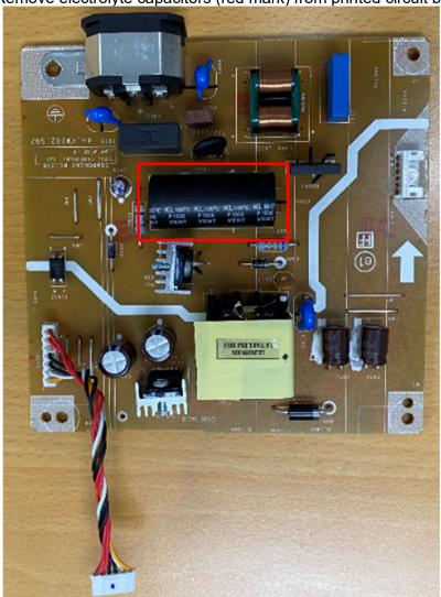
S20-1 Cut the glue between bulk cap. and PCB with a knife
