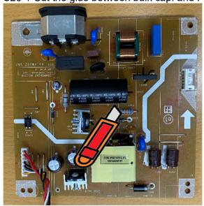
S20-2 Ensure cutting path within the glue, don't touch bulk cap. or PCB
