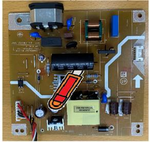
S20-3 Take out bulk cap. pin solder with soldering iron and absorber
