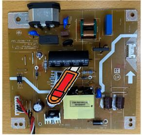
S22-3 Take out bulk cap. pin solder with soldering iron and absorber
