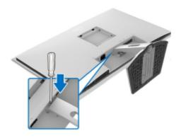
Once the latch is released, slide the stand assembly away from the monitor
