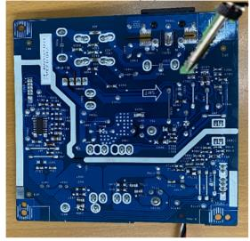
S22-4 Lift the bulk cap. up and away from the PCB
