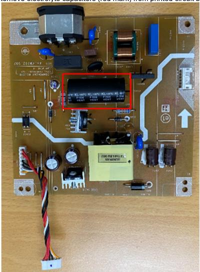
S22-1 Cut the glue between bulk cap. and PCB with a knife
