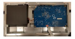
S19 Disassemble the little Mylar from Main
