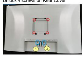
(Screw Torque: RC screw: 8.5±1.0kgf Stand screw: 4~5kgf)
