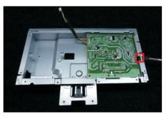
Take a interface board, connect a LVDS cable to the connector of the interface board, then connect the cable of the power board to the connector of the interface board. Turn over the interface board and locate it into the bracket. Use a Philips-head screwdriver to tighten 5pcs screws for locking the power board and interface board.
