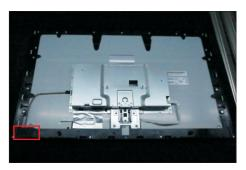
Take 1pcs rear cover, put down the rear cover and push the rear cover on the positions marked as the picture below shown for mechanisms engagement.
