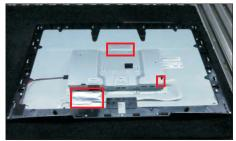
Use a Philips-head screwdriver to remove 18pcs screws for unlocking the middle bezel.
