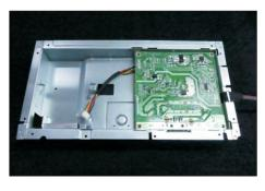
Remove the interface board and power board from the bracket chassis module carefully, and disconnect all the cables.
