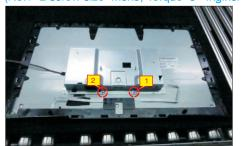
Take away the middle bezel, and put it on a fixture. Use a Philips-head screwdriver to remove 3pcs screws for unlocking the function key board, and then tear off the tapes for releasing the key cables. (No.1~3 screw size=M2x2.4, Torque=0.8±0.2kgfxcm
