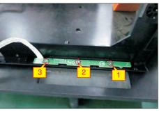
Tear off the tape, then lift up the panel module with the bracket chassis for releasing the front bezel away from the panel module.
