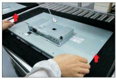
S11 Unplug the LVDS cable from the connector of the panel module by pushing the earing-locks.
