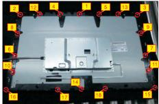
Use a Philips-head screwdriver to remove 2pcs screws for unlocking the bracket with panel module.
