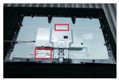
Use a Philips-head screwdriver to remove 18pcs screws for unlocking the middle bezel.
