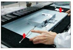
S11 Unplug the LVDS cable from the connector of the panel module by pushing the earing-locks.
