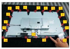
Use a Philips-head screwdriver to remove 2pcs screws for unlocking the bracket with middle bezel, to remove 2pcs screws for unlocking the bracket with panel module.
