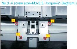
Connect the panel lamp cable to the connector of panel, then cover the connector with 1pcs acetate tape. Plug the key cable to the connector of the board. Paste 1pcs aluminum foil to fix the key cable and LVDS connector.
