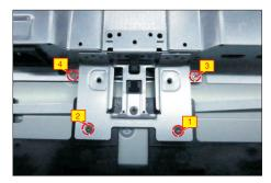
Use a Philips-head screwdriver to remove 13pcs screws for unlocking the middle bezel with the assembled unit.
