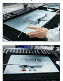
Take a function key board and a middle bezel, then fix the middle bezel with a fixture, and locate the function keyboard into the hooks of the bezel. Use a Philips-head screwdriver to tighten 3pcs screws for locking the function key board with the middle bezel. (No.1~3 screw size=M2x2.4, Torque=0.8±0.2kgfxcm
