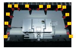
Take away the middle bezel, and put it on a fixture. Use a Philips-head screwdriver to remove 3pcs screws for unlocking the function key board with the middle bezel, and then tear off the tapes for releasing the key cables.
