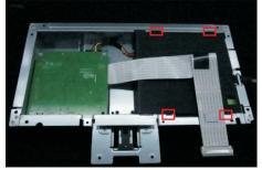
Panel preparation: Take out 1pcs panel module from the carton, then remove the protective film by tearing off the tapes, and then examine the panel surface according to inspection criteria. Turn over the panel, and then place screen faced down for later assembling.
