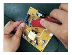
S18-3 Cut into the bottom of bulk cap. and pullit up carefully.
