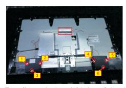
Tear off 1pcs aluminum foil (refer to S7) and then remove the two speakers. Use a Philips-head screwdriver to remove 5pcs screws for unlocking the middle bezel with front bezel.
