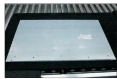
Remove the Mylar from the hooks of the bracket chassis module.
