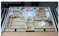
Take out of the molded pulp with base, riser and cover from the carton, then take out the monitor from the EPE bag and put it on a protective cushion.
