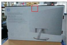
S2 Take out all of the accessories including QSG, HDMI cable, power cable, CD&user's manual, stand base, stand riser and EEI label from the carton. (Note: It depends on whether users returning the accessories)
