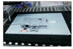
S14 Take away the bracket chassis module and then put the bracket chassis module on a protective cushion.
