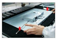
S13 Unplug the LVDS cable from the connector of the panel module by pushing the earing-locks.
