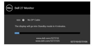
This box also appears during normal system operation, if the video cable becomes disconnected or damaged. Turn Off your monitor and reconnect the video cable; then turn On both your computer and the monitor.
