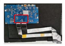
Remove electrolyte capacitors (red mark) from printed circuit boards
