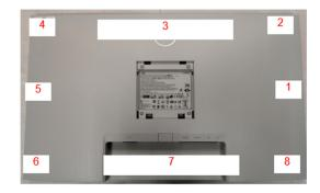
S7 Tear off all adhesive tapes from backlight wire and SPK wire
