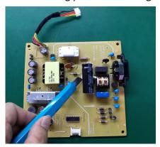
S1 -3 Cut into the bottom of bulk cap. and pull it up carefully
