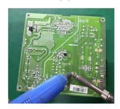
S1 -5 Lift the bulk cap. up and away from the PCB
