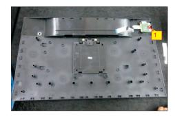
Use a proper tool to release the function key cable from the connector, then pull the function key cable high for releasing the function key cable.
