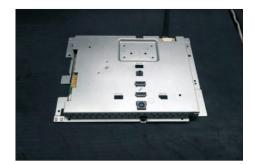
Turn over the bracket chassis module. Use a Philipshead screwdriver to remove 5pcs screws for unlocking the main board.
