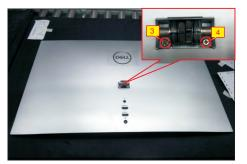
Use a proper tool insert the gap of the rear cover top side (marked 1) as the following picture to release the rear cover, then wedge your fingers between the rear cover and the panel to release the rear cover, then use one hand to press the panel module, the other hand to pull up carefully the rear cover in order of arrow preference 1~3 for unlocking mechanisms of rear cover, and then remove the rear cover carefully.
