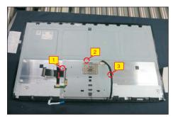
Use a Philips-head screwdriver to remove 4pcs screws for unlocking bracket, move away the bracket and then remove 1pcs screw for unlocking the front bezel from the panel module, and then remove the front bezel carefully.
