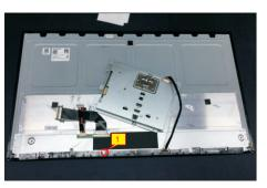
S10 Put the front bezel with function key board into a fixture, tear off the mylar, then use a Philips-head screwdriver to remove 3pcs screws for unlocking the function key board with front bezel.
