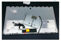
Adjust the bracket to make it with the panel module firmly attachment. Use a Philips-head screwdriver to tighten 4pcs screws for locking bracket with front bezel and panel module.
