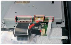
Use a Philips-head screwdriver to remove 3pcs screws for unlocking bracket with panel module.
