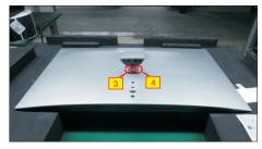
Take a base to assemble it with stand, then use a Philips-head screwdriver to tighten 3pcs screws for locking the stand with base. Take 1pcs decoration strip, tear off the adhesive paper and stick it on the correct position as the picture below shown.
