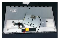
Put the front bezel with function key board into a fixture, tear off the mylar, then use a Philips-head screwdriver to remove 3pcs screws for unlocking the function key board with front bezel.
