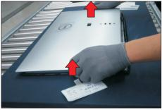
Tear off 2pcs double-faced tapes on the left and right side of the middle bezel, then tear off 2pcs aluminum foil to release the panel lamp cable and LVDS connector.
