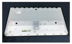
Stick 1pcs mylar tape on the correct position and then use a Philips-head screwdriver to tighten 3pcs screws for locking the panel module, then connect 1pcs LVDS and 1pcs panel lamp cable into the connectors. Stick 2pcs double-faced tapes on the specific position of the panel module as the picture below shown.
