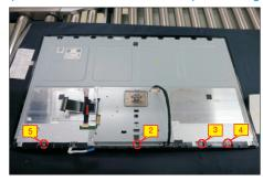
Use a Philips-head screwdriver to tighten 3pcs screws for locking bracket with panel module, then use a proper tool to connect the LVDS cable, panel lamp cable and function key cable to the connectors of the main board.
