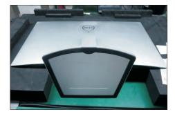
Lift up the stand, then use a Philips-head screwdriver to remove 2pcs screws for unlocking the whole unit including stand and base, then remove the stand and base. Use a Philips-head screwdriver to remove 2pcs screws for release the hinge cover.
