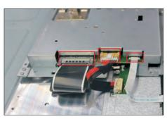
Use a Philips-head screwdriver to remove 3pcs screws for unlocking bracket with panel module.
