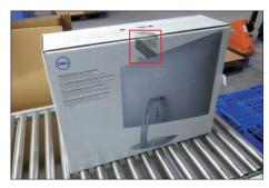
Take out the QSG from the catron, and then take out the Paper-Top with other accessories including user's manual, HDMI cable, power cable, power adapter and other packing materials from the carton. (Note: It depends on whether users returning the accessories)
