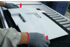
Tear off 3pcs aluminum foils, then disconnect speaker's cable away from the connector of the interface board. Use a Philips-head screwdriver to remove 6pcs screws for unlocking the two speakers.
