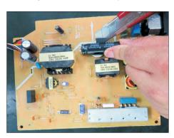
S22-2 Ensure cutting path within the glue, don't touch bulk cap. or PCB.
