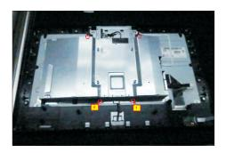
Disconnect the LVDS cable and 1pcs panel lamp cable away from the connectors of the panel module, then take away the bracket chassis module and then put the bracket chassis module on a protective cushion.
