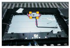
Tear off the camera glass, then release the back cover away from the unit, then use a Philips-head screwdriver to remove 2pcs screws for unlocking the holder board with the camera from the bracket unit, and then disconnect the connective cable from the camera. Tear off camera from the holder board.
