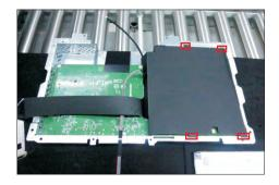
Use a Philips-head screwdriver to remove 8pcs screws for interface board and power board. Release the connective cable and panel lamp cable from the hooks of the bracket
