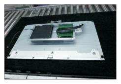
S12 Remove the Mylar from the hooks of the bracket chassis module.
