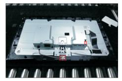
Paste 1pcs aluminum foil to cover the LVDS connector, then paste 1pcs aluminum foil to fix bracket chassis as the picture below shown.
