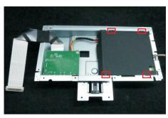
Panel preparation: Take out 1pcs panel module from the carton, then remove the protective film by tearing off the tapes, and then examine the panel surface according to inspection criteria. Turn over the panel, and then place screen faced down for later assembling.
