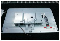
Take away the bracket chassis module and then put the bracket chassis module on a protective cushion.
