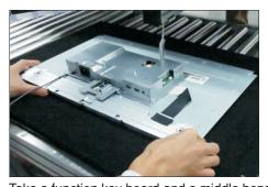
Take a function key board and a middle bezel, then fix the middle bezel with a fixture, and locate the function keyboard into the hooks of the bezel. Use a Philips-head screwdriver to tighten 3pcs screws for locking the function key board with the middle bezel. (No.1~3 screw size=M2x2.4, Torque=0.8±0.2kgfxcm
