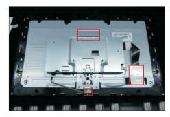
Use a Philips-head screwdriver to remove 16pcs screws for unlocking the middle bezel.
