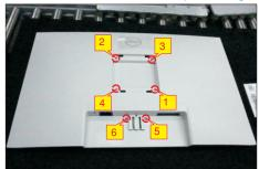
Stick 2pcs labels on the specific positions as the picture below shown. Take 1pcs stand riser and 1pcs stand base, assemble the stand base with stand riser, then rotate the screw clockwise to lock the stand base and stand riser. Insert the stand-riser into monitor groove until it snaps into its place.
