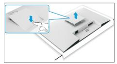
Use a Philips-head screwdriver to remove 6pcs screws for unlocking mechanisms.
