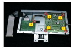
Take a mylar to insert the hooks of the bracket to cover the power board.
